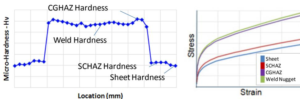
Figure 7: Weld Hardness Profile and Scaled Stress Strain Curves
