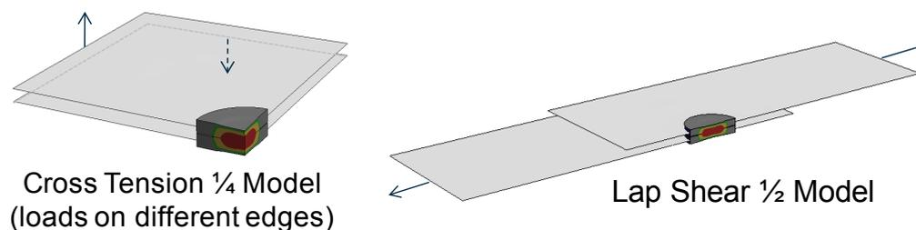
Figure 6: Cross Tension and Lap Shear CAE Model Configurations
