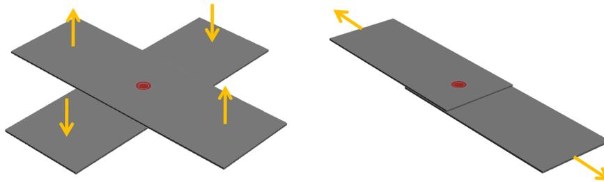
Figure 3: Cross Tension and Lap Shear Test Configurations
