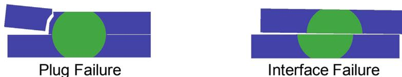
Figure 4: Spot Weld Failure Modes
