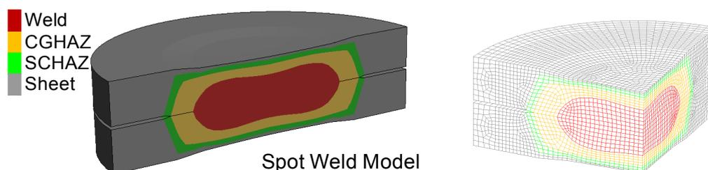
Figure 5: CAE Model of Weld, CGHAZ, SCHAZ and Adjacent Sheet
